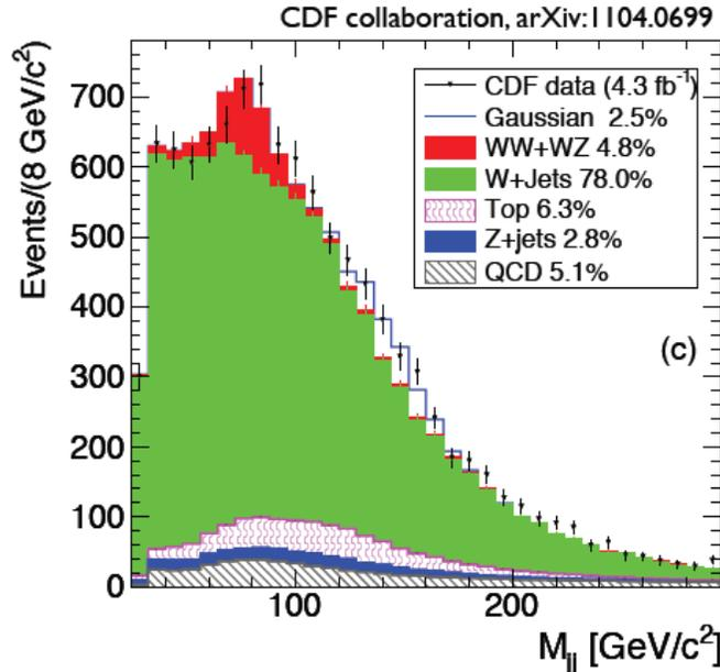
The figure above shows the production of a W boson and two parton jets with the interesting physics showing up as only a small deviation from the theoretically predicted background of the null hypothesis. Clearly, an accurate prediction of the background is critical to verifying physics such as the Higgs boson. In order to predict this background, we look at a given process and identify the subprocesses that contribute to it.
